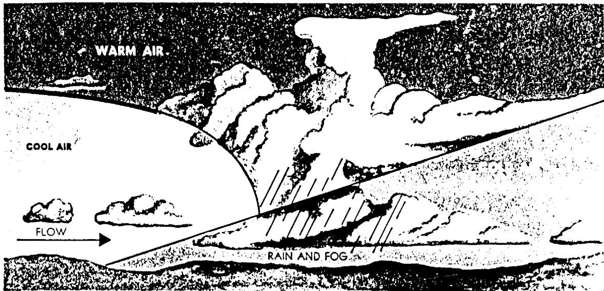
FIGURE 73. A warm front occlusion lifting warm, moist, unstable air. Note that the associated weather is complex and encompasses all types of weather associated with both the warm and cold fronts when air is moist and unstable.
